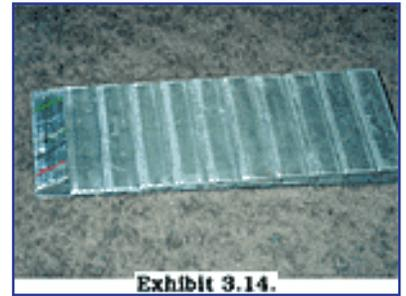
Schools should initially run this test to accept the equipment and on a regular basis, such as once a month, for validating that the system is still performing well. Any significant decrease in the number of wavy wires that are visible may indicate that the unit needs repair.
