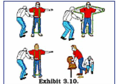
1. Ask the scannee to place all carried items, plus any caps or headgear on a table (procedures for manual search of baggage are not covered in this text). The scannee should stand with his or her feet about 18 inches apart, facing away from the table and about 2 feet in front of it. Footprints outlined on the floor or drawn on a mat can greatly help position the scannee properly. Ask the scannee to hold his or her arms out to the sides, parallel to the floor.
