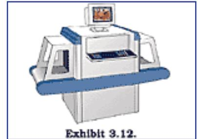
Generally, between 10 and 20 items per minute can be examined using an x-ray baggage scanner. As many as 30 items per minute can be effectively scanned if most of the items are benign, i.e., contain no obvious metal items larger than a coin or button, none of which are touching in the image. Dense clutter within a bag will necessitate that bag being pulled off the conveyor to be manually searched.
